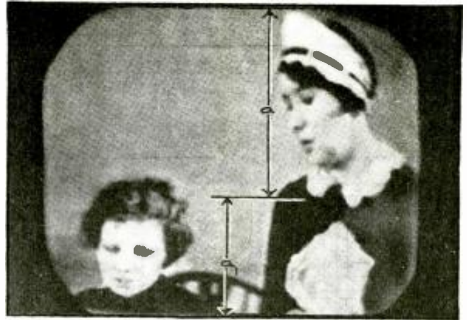
Fig. 8. This illustrates the unpleasant effect secured with a non-linear vertical scan. The distances a and a1 normally should be equal. The image is badly distorted.
