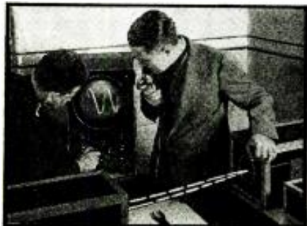
Westinghouse engineers check the infra-red ray talking beam over which spectators at the New York World's Fair will talk and "see" their voices on a C.-R. oscilloscope.
