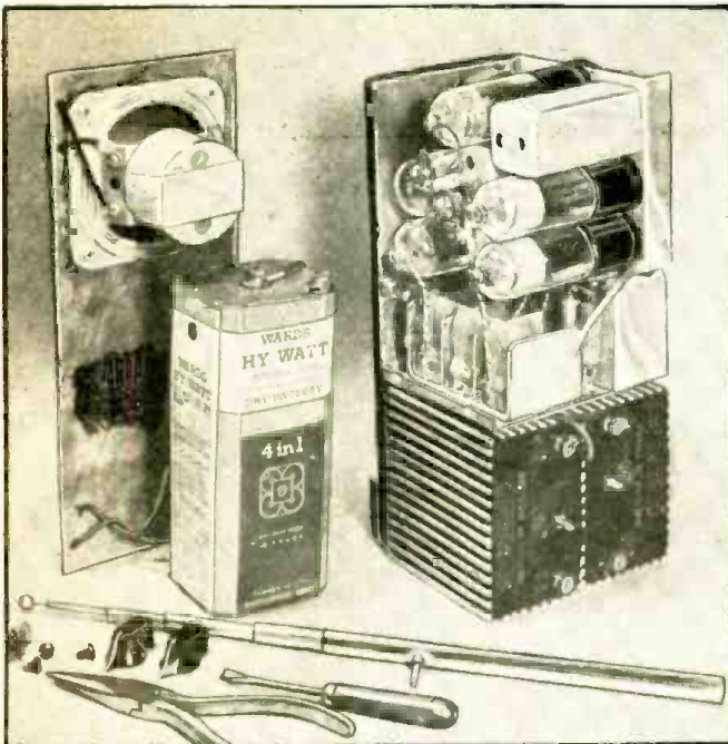
Fig. B. The "innards" of the Lunchbox Portable. One No. 6 drycell will run the set for months. Note the P.-M. dynamic speaker above the cell; and note the telescoping fishpole-type antenna which plugs into the front panel and extends to 45 ins.
