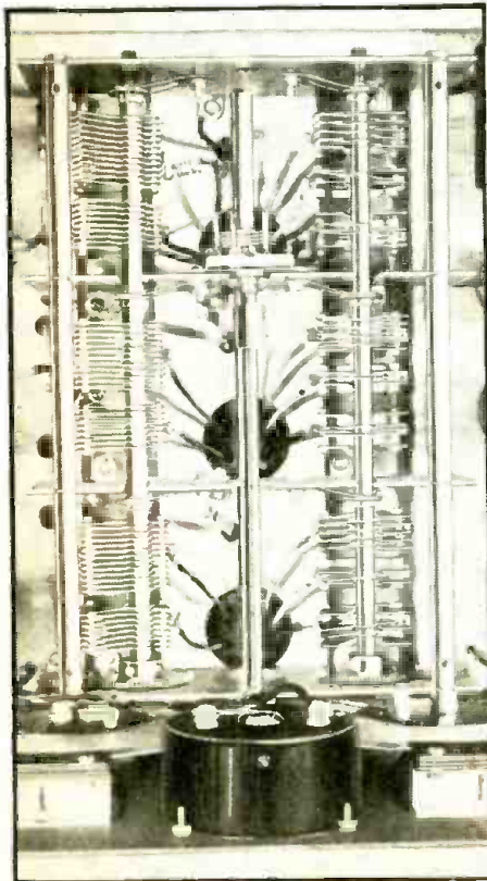
Fig. C. View, showing main tuning and bandspread condenser assemblies. The small condenser in the center, with the extended shaft, is the antenna compensator. Note that there are 3 rotor contacts for each section. These are inlaid, silver-to-silver contacts. The rotors of the 2 large condenser assemblies are hung on ball bearings—one at each end.
