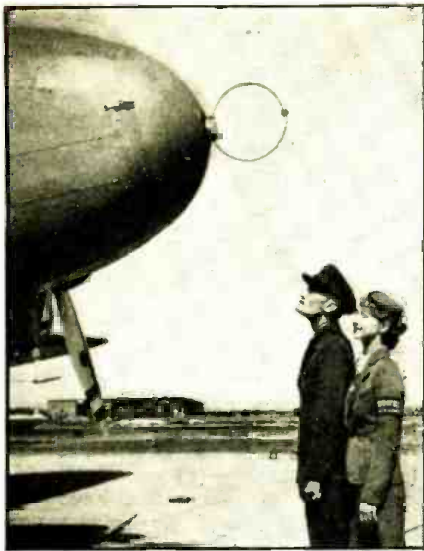
The new "anti-static" loop antenna that permits constant reception of directive radio beam signals.
