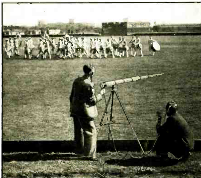
New W. E. "machine-gun" mike, at Polo Grounds in N. Y. C., picking up music of a band (not shown in photo) on which it is trained; music of brass band shown above is not heard since only bass notes can be heard off-beam.
