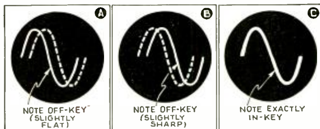
Fig. 2. The vocalist (or instrumentalist) provides vertical-sweep-circuit frequencies by singing (or playing) into the microphone; which is connected through an amplifier to the "resonoscope." "Drifting" of the waveform left or right from a central position indicates, respectively, "flat" or "sharp." Radio-Craft editors have witnessed demonstrations of this amazing device which prove quite definitely that even professional singers and musicians seldom realize when they are off-key. In fact, other tests show, skilled instrument tuners may vary 1/3-cycle from fundamental notes; but this new, uncanny, "electronic robot" is precise to about 0.002 per cent!
