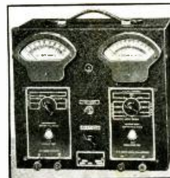
Test unit; wide-range scales—to 20 meg., 1,000 V. D.C., 800 V. A.C. 16 mf. and 500 ma. (1436)
