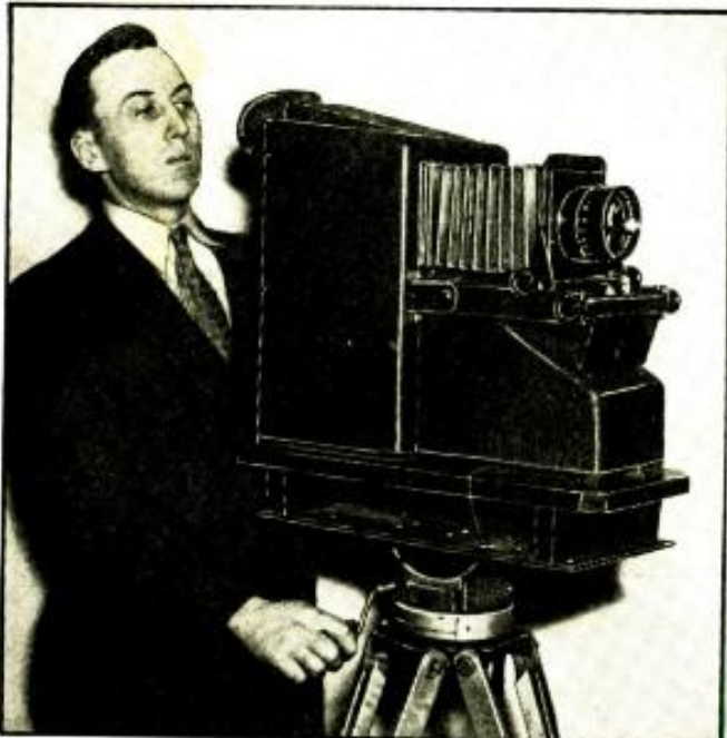
Fig. B. Charles Stec operating a Philco 441-line, television-transmitter "camera."
