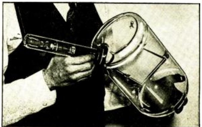
Fig. D. This "camera tube" will televise even the second-hand of a watch!
