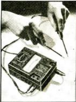
A "megger" cross-coil moving system is used in this meter (range—to 0.2-meg.). (1421)
