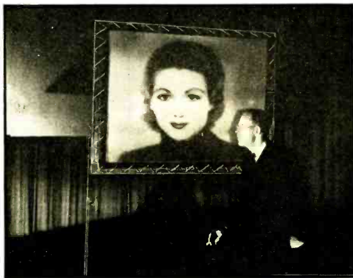
Fig. A. Here is a view of Dr. Law and the projection type cathode-ray television image he obtained on a 3 x 4 ft. screen.
