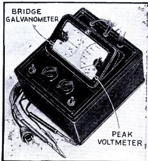
This V.T. voltmeter has linear scale readings. It is the first instrument of its kind to bring to the technician the precision facilities of both the bridge-type galvanometer and the peak voltmeter, in a test unit rugged enough for use in portable service. Note that the meter needles indicate vertically. (1126)
