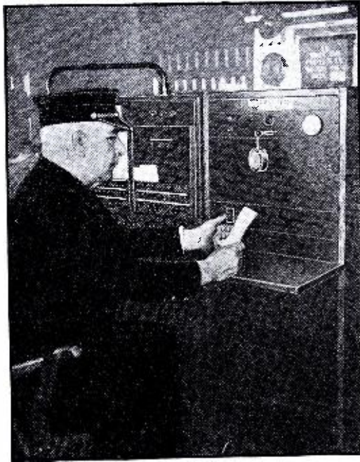
Above, the unit installed in every Fire Station—it consists of an alarm and an amplifier.
