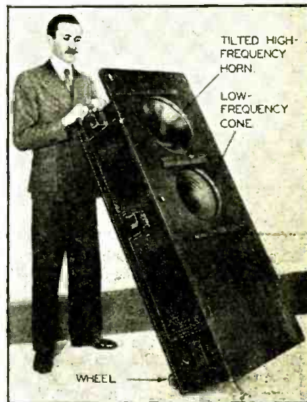
Fig. E. The amplifier and dual-speaker unit for the reproduction of high-fidelity wired sound. Wheels and a handle permit easy transportation.
