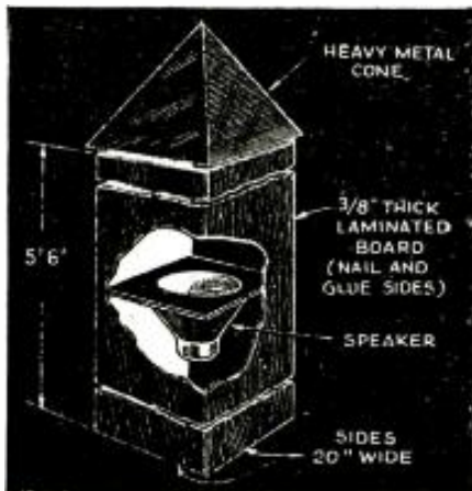
Fig. 2. Constructional details of the "sound columns" used to build up response in the "dead spots" caused by insufficient speaker coverage. The metal top deflects the sound down to the audience.
