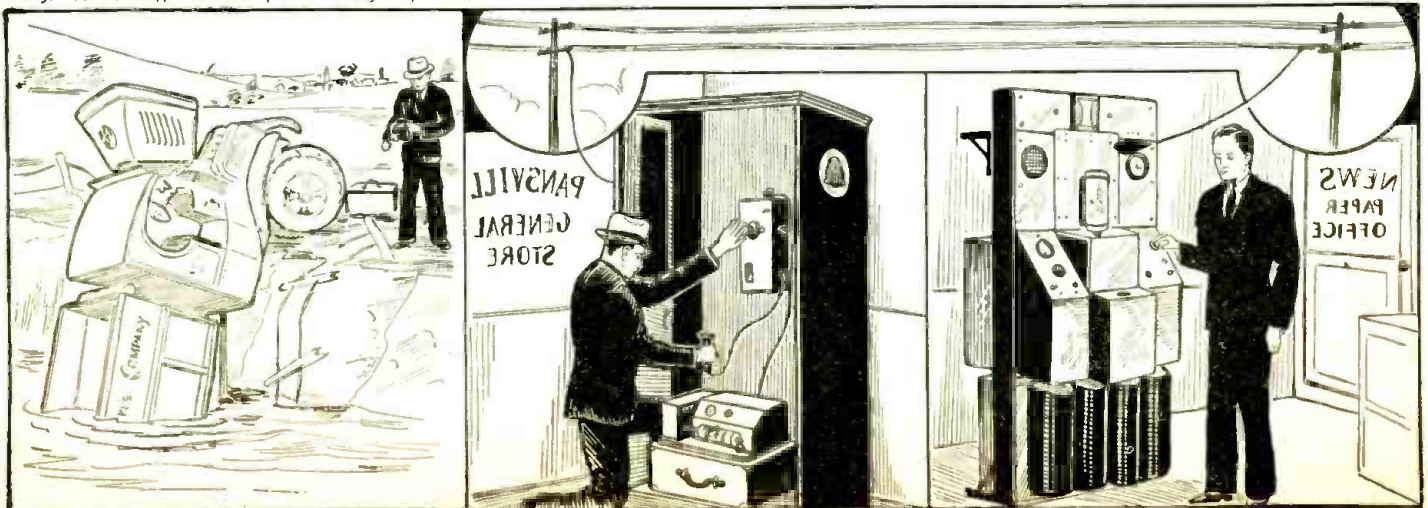
Fig. 1. The 3 steps. First the picture is taken, then developed; second, it is sent over the line; and third, received (as shown in Fig. D) at the newspaper office.
