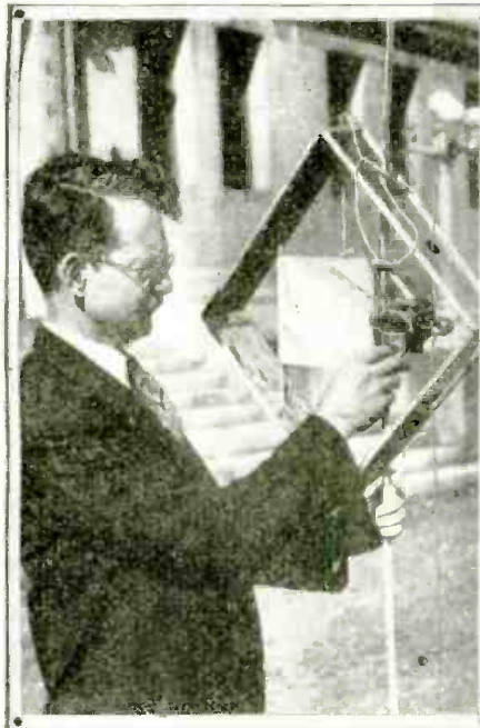
↑ be used in conjunction with the Weather Bureau in Meteorological experiments. Tests have been made which show that this equipment, which weighs less than 2 lbs., can be heard at a distance of 80 miles, and as high as 14 miles. The transmitter operates on 5 Meters. (Harris & Ewing)
