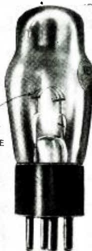
HAIR-FINE BALLAST RESISTANCE WIRE
