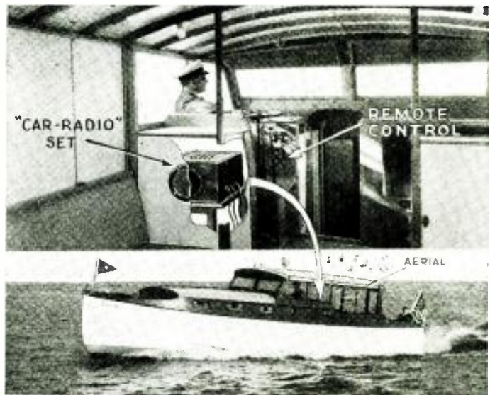
Fig. A. The remote control, like in a car, can be mounted on the dash.
