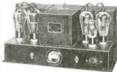
Fig. A, below. The extreme compactness and neatness of this 100-watt power stage, also layout, are clearly shown.
