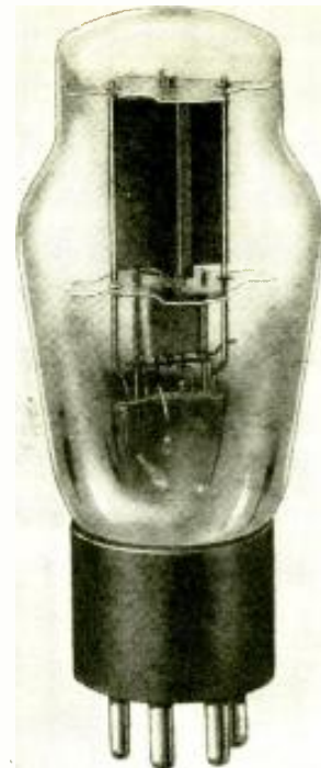
The 2B6—an improved Triple Twin.
