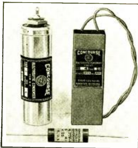
A photograph illustrating representative electrolytic condensers. The one in the foreground has a capacity of about 5 mf. suitable for bypassing purposes.
