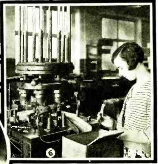
(6) Automatic Flare Machine —Long lengths of glass tubing are placed in the revolving chucks which are shown at the top of this machine. These chucks feed the glass tube, at a predetermined, desired length, into a number of gas flames. There are eight sets of gas flames which the tube passes through from the time the operation starts until the flare is finished. Each different position is accompanied by an increase of temperature of the flame acting upon the glass tubing as the process develops. At the position shown directly before the operator is a revolving steel flare cutting disc.
