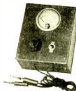
The circuit and outward appearance of the Scott continuity meter, useful for many purposes.
