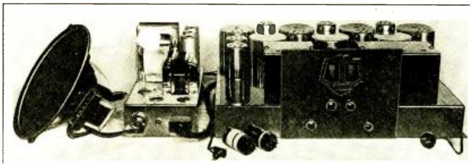
Fig. B From right to left, tuner, amplifier-pack, and reproducer; showing the connecting cables which give flexibility of placement. Note the complete shielding and strong construction.
