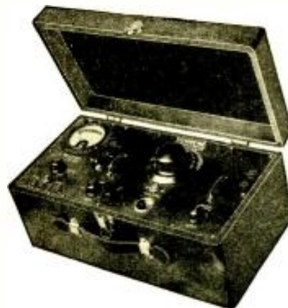
The Supreme "Model 70" oscillator in its carrying case; with the output meter at the left.
