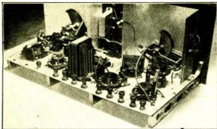
Mr. Ulrich's remodeled "Super-Wasp," with tubes, coils and rear shields removed to show the placing of parts. The R.F. stages are seen at the right; detector and oscillator left; audio between.
