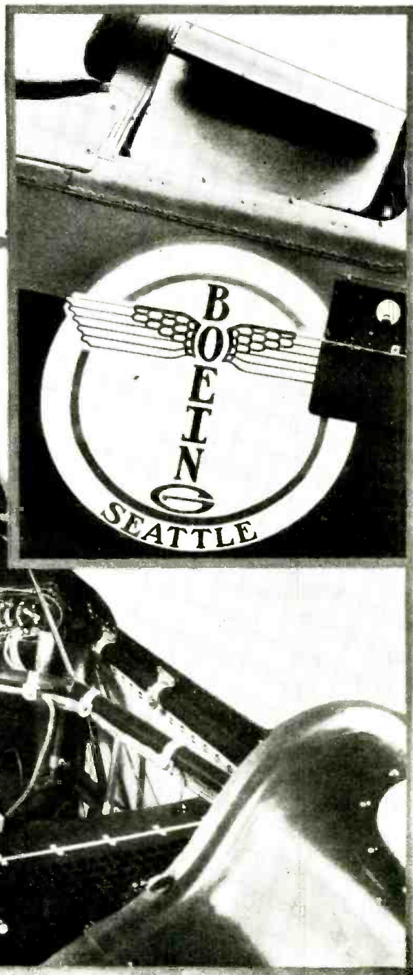
At the right, the side of a mail-passenger plane, showing the small door beside the second compartment, through which the station operator tunes the set before a flight is commenced. Directly behind this rises a streamlined dual antenna mast. Below, a view of the compartment, showing the receiver and transmitter, with their shielded cabin. (Photos courtesy Boeing System.)
