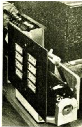
A close-up view of the Carter "Electro-Automatic" tuning selector.
