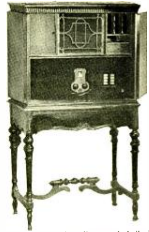
The Carter automatic radio control, built into a standard receiver console.
