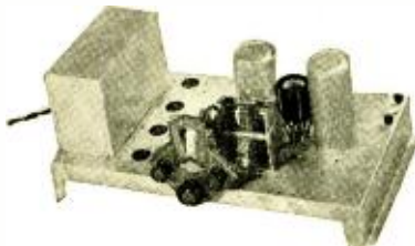
Chassis of the "Round-the-World Six," a 17-meter factory assembled receiver.
