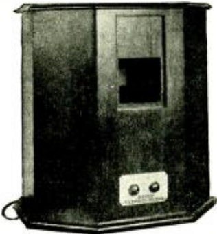
An early American television unit incorporating scanning disk, neon lamp, television frequency amplifier and power supply.
