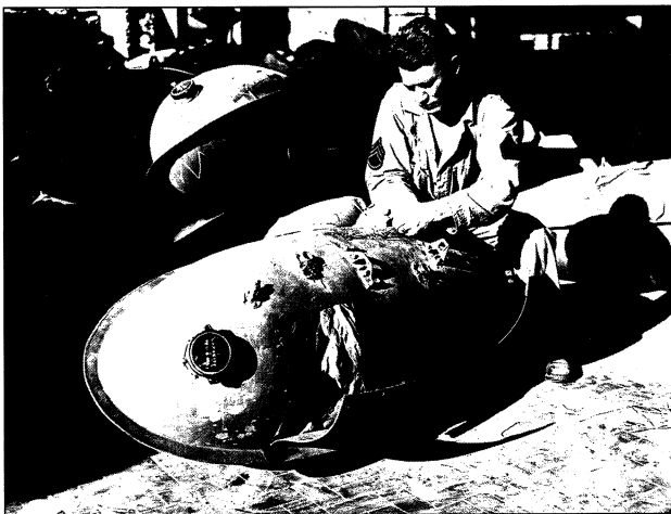
FIGURE 7: MODIFIED DETACHABLE FUEL TANKS. A detachable fuel tank is shown, modified to drop supplies to friendly troops. Records reveal that parachutes were used to drop rations to the lost battalion. The author was unable to obtain details on how this was accomplished. Photo courtesy of Quartermaster Corps Museum, Fort Lee, Va.
