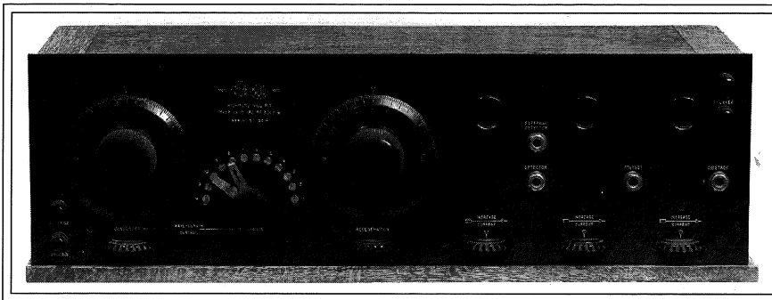
◆ Photo 3. The CR-9 has two stages of audio amplification and is able to drive a horn loudspeaker.
