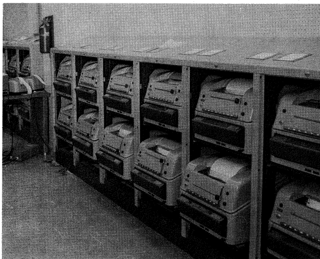
Model 28 Receive-only Page Printers used to produce hard copy of messages received from points all over the world.
