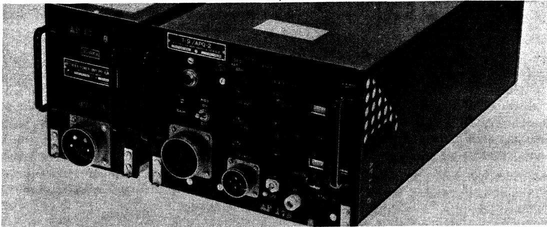
Fig. 4 - One of a Line of Standardized Radar Jammers; Known as "RUG", This Set Tunes from 200 to 550 Megacycles.
