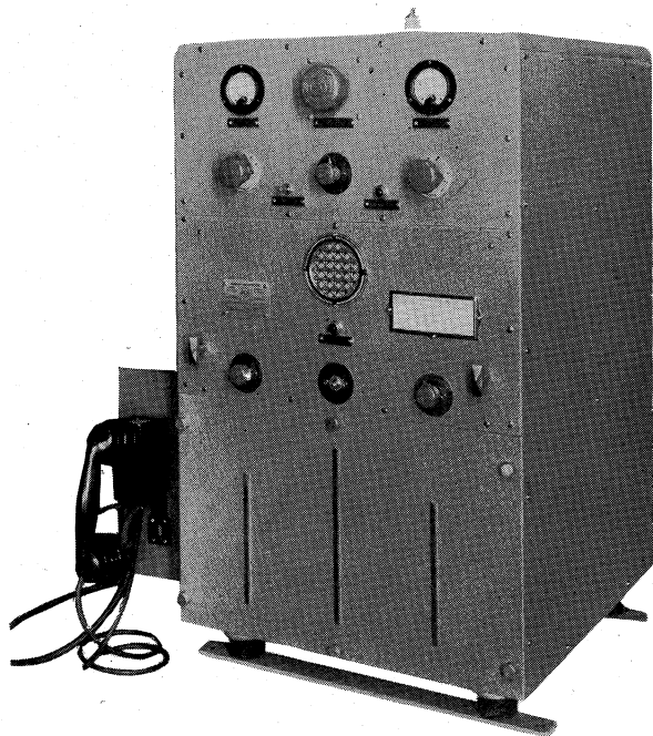
Fig. 7—Radio equipment, 75 watts in power.
