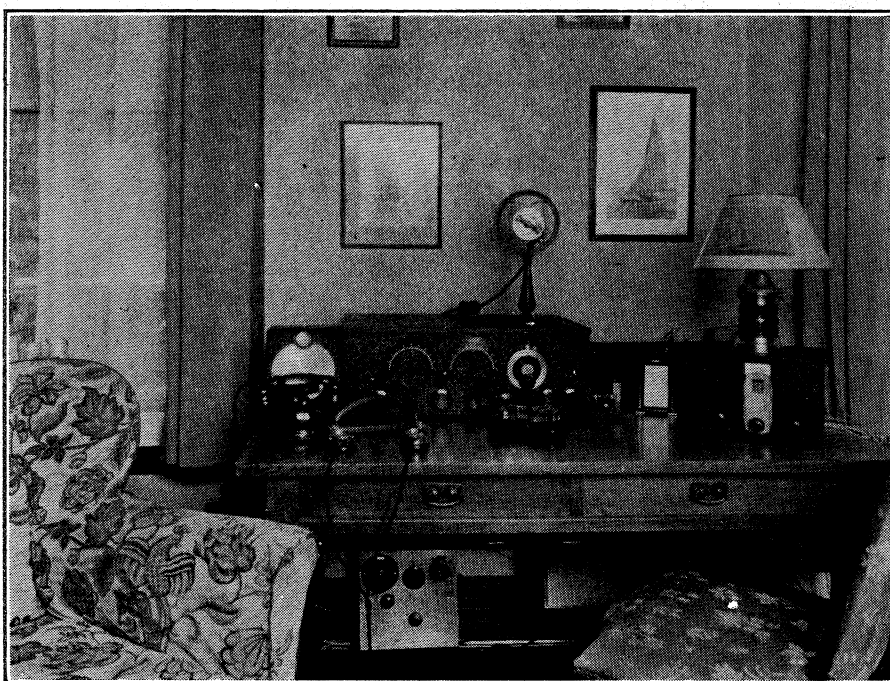
Receiver, station "W2AG," C. R. Runyon, Yonkers, N. Y., 1933. Note—single signal short wave superheterodyne center, and super-regenerative 5 meter receiver on the right. Randy Runyon was the first amateur to develop and use the single signal superheterodyne receiver, which is now the last word in C. W. reception.
