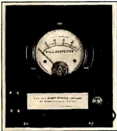
Front view of output meter.
