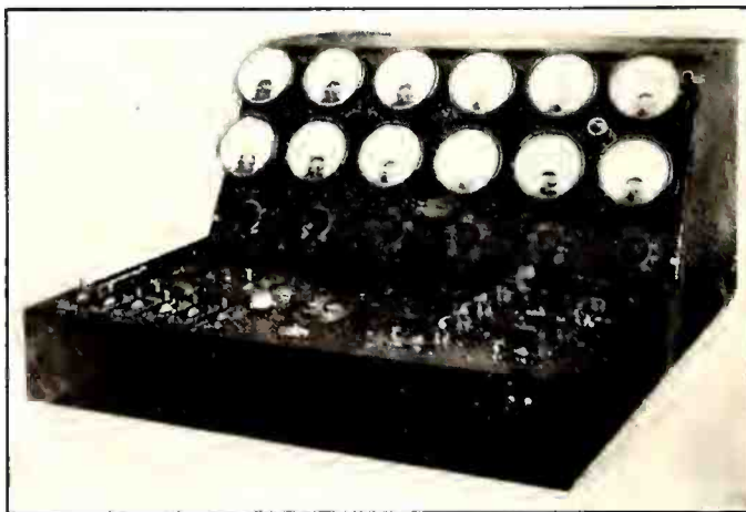
This elaborate tube-tester was designed by Westinghouse. It is intended especially for manufacturers' use.
