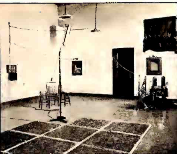
The two pictures above and the one below show views of the apparatus used by F. R. Watson, of the University of Illinois, in his tests on acoustic material. The results of this work appeared in bulletin No. 172 published by the University. Above is shown the reverberation room.
