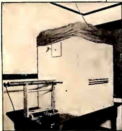
A Rayleigh disc having a period of vibration of 15 seconds was housed in the box shown above. The disc was 1.2 cm. in diameter, 34 mg. in weight, and was suspended by a quartz thread about 15 cm. long.
