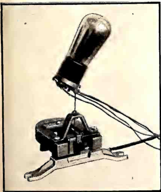
A vibrator unit employed in tests to determine the conditions under which vacuum tubes are microphonic.
