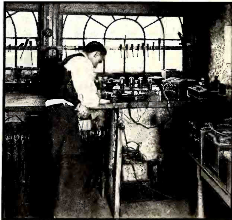
Fig. 5—Making a continuity test on a radio receiver under ideal conditions with plenty of daylight and the proper test equipment.
