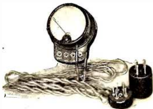
A HANDY A.C. VOLT-METER AND TEST PLUG
