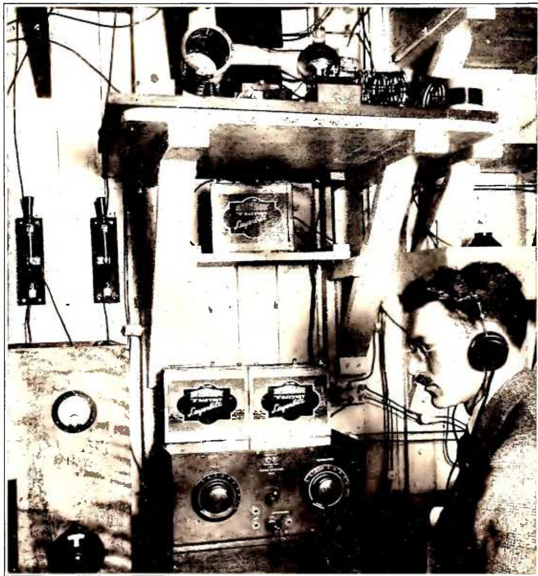
THE RADIO EQUIPMENT ABOARD THE "MORRISSEY" IN THE FAR NORTH Edward Manley, of Marietta, Ohio, is shown before the radio apparatus aboard the Putnam-Baffin Island expedition. The Morrissey , known to the short-wave code world as VOQ has a generator-powered short-wave transmitter, a battery-powered transmitter using a UX-852 tube (on the top shelf), a short- and long-wave receiver, and a portable battery-operated transmitter. Signals from VOQ have been clearly heard at the short-wave laboratory of RADIO BROADCAST and occasional radio dispatches from the expedition have appeared in the New York Times
