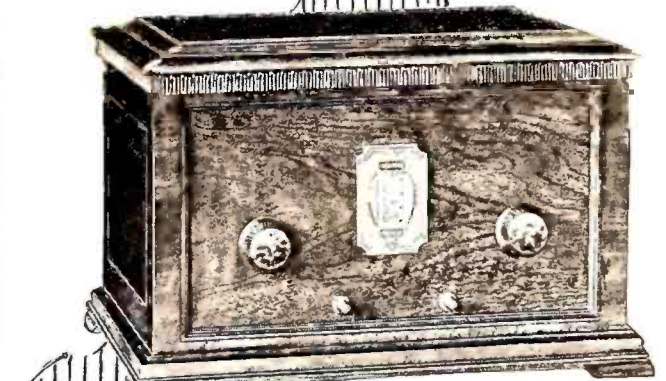
MU-RAD Two t. r. f. stages, detector, and three audio stages are included in this receiver. The audio stages, all of the double-impedance form, give uniform response between 30 and 5000 cycles, according to the manufacturers. Single-control tuning is featured. Price $98.00. In a console, equipped for complete a. c. operation, the receiver sells for $265
