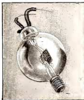
The first Radio Tube in the World, 1906, from which has sprung the present gigantic radio industry. The device through which natural sounds audible to the human ear were transmitted by radio for the first time.
