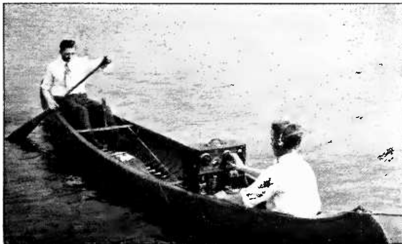
In the canoe the antenna is held in place by two small insulators and the kite is somewhere above. The "ground" connection is made by merely dropping a brass rod attached to the ground wire over the side of the canoe
