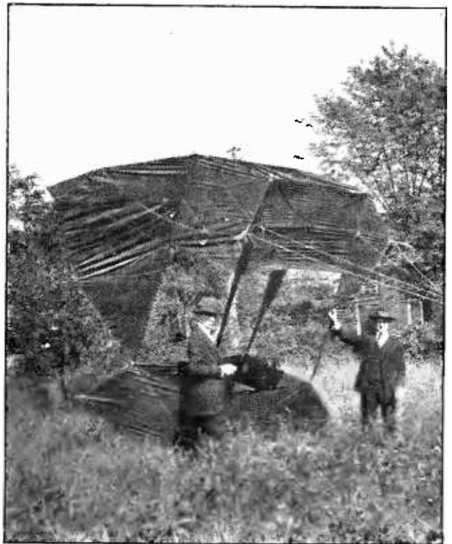
This is an ex-service, man-carrying kite now used to carry an antenna. Some idea of its size may be had by comparing it to the men who are holding it. A suitable kite-string may be made from a stout clothes line
