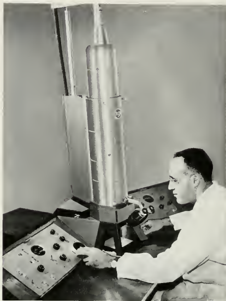
A leading electronic contribution to medicine is RCA's electron microscope, shown here in operation at Armed Forces Institute of Pathology, Washington.
