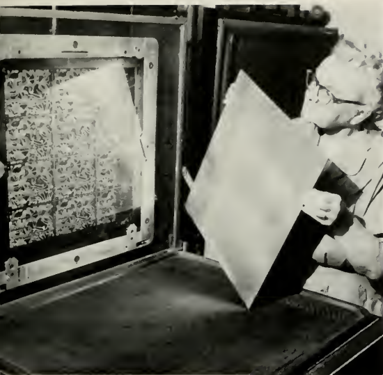
3. Image is printed on a plastic board with a veneer of photo-sensitized copper. Here the board is inserted in the printer, against the glass negative, for exposure.
