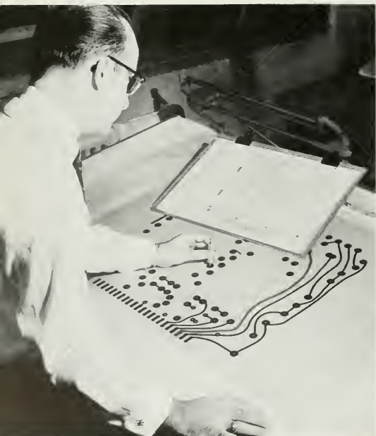
1. Process begins with preparation of a large production photo-master of the original circuit drawing. Here photo-master is copied from small drawing at top.
