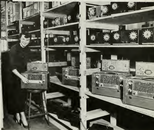
Globe-girdling "Strato-World" portables and table model clock radios (right) are checked for performance, life-span and overall dependability.
