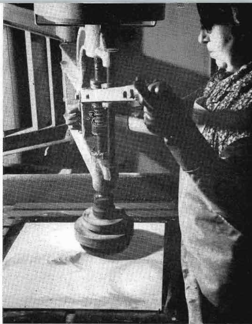
A copper-clad sheet of plastic, on which electronic circuits will be printed by photography, is highly polished before the light-sensitive emulsion is applied.
