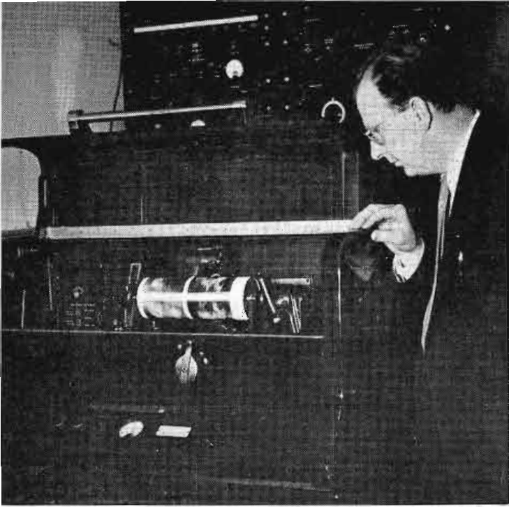
Charles H. Colledge of NBC's Public Affairs Department inspects the transmitting unit of a Mufax transmitting unit from which still pictures were sent direct to New York by transatlantic radio.
