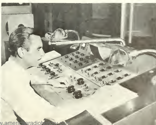
AT THIS CONSOLE THE MIXING ENGINEER FOLLOWS HIS CUES AND COMBINES SOUND EFFECTS, WORDS AND MUSIC IN PROPER RELATION FOR INSCRIBING ON THE FILM.
