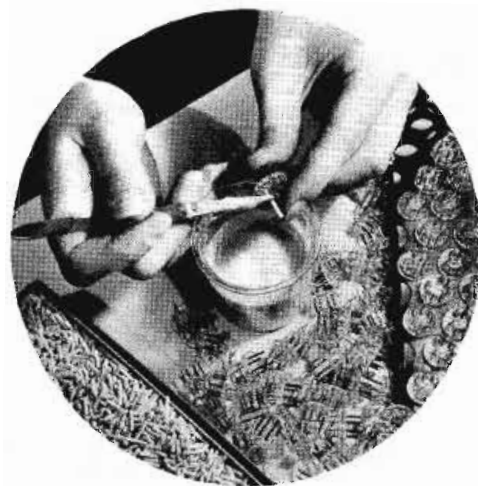
CEMENTING CERAMICS INSULATION IN MINIATURE TUBE MANUFACTURE CALLS FOR STEADY HANDS AND KEEN EYESIGHT.
