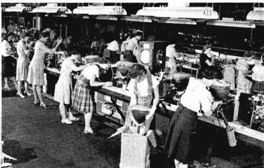
TELEVISION RECEIVERS WITH KINESCOPE PICTURE TUBES IN PLACE MOVE DOWN PRODUCTION LINES AT RCA VICTOR ON THEIR WAY TO THE TESTING CHAMBER, THE LAST STOP BEFORE SHIPMENT.
