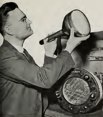
E. EBERHARD OF RCA TELERAN ENGINEERING DEPARTMENT HOLDS ONE OF THE NEW HIGH-INTENSITY TELERAN TUBES. BELOW IS A TYPICAL TELERAN IMAGE AS IT APPEARS ON THE TUBE FACE.
