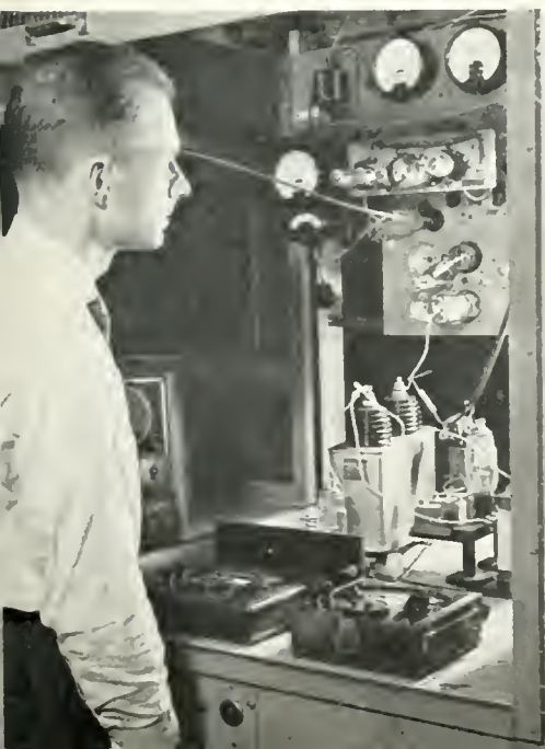
DR. H. B. DEVORE MAKES A PRELIMINARY ADJUSTMENT ON THIS HIGH-VOLTAGE TEST CAGE, IN WHICH THE TUBE IS FINALLY CHECKED IN A COMPLETE CIRCUIT.
