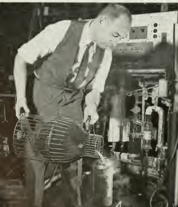
LIQUID AIR, TEMPERATURE 313 DEGREES BELOW ZERO, FAHRENHEIT, IS USED BY J. BURNETT TO IMPROVE THE VACUUM IN A TUBE WHEN IT IS COMPLETED. BELOW, H. A. FINKE TAKES PERFORMANCE DATA ON A BEREARCH TUBE AS IT IS PUT THROUGH ITS PACES IN AN ELABORATE SERIES OF ELECTRICAL TESTS.
