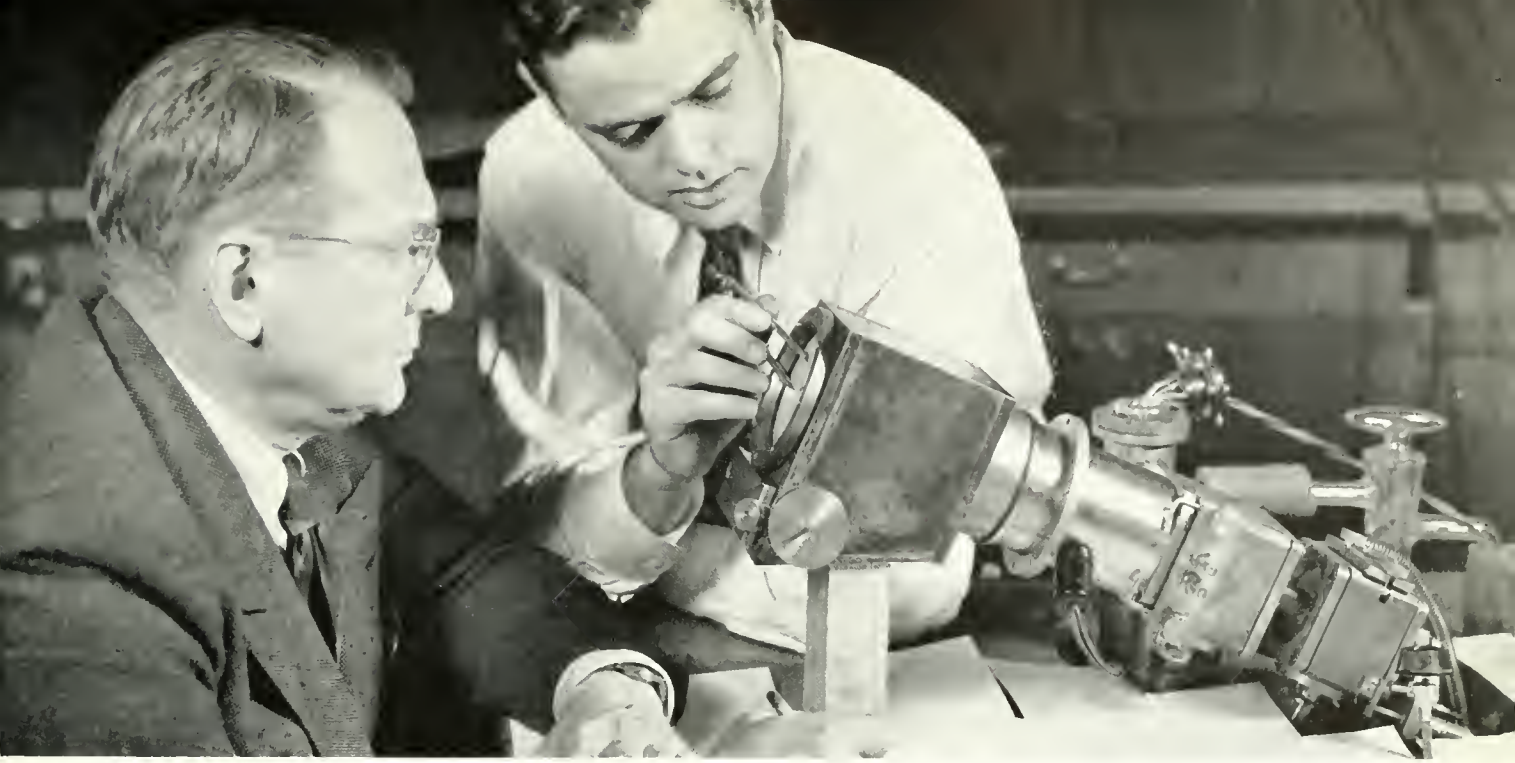
DR. V. K. ZWORYKIN (LEFT) AND DR. JAMES HILLIER OF RCA LABORATORIES EXAMINE THE NEW DESK-SIZE RCA ELECTRON MICROSCOPE. DEVELOPMENT OF THE INSTRUMENT WAS ANNOUNCED IN NOVEMBER AT CHICAGO. IT IS CAPABLE OF THE SAME HIGH DEGREE OF RESOLUTION AS RCA'S STANDARD MODEL.
