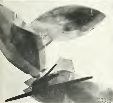
CRYSTALS OF ALUMINUM OXIDE MONOHYDRATE, AS SEEN BY THE ELECTRON MICROSCOPE.
