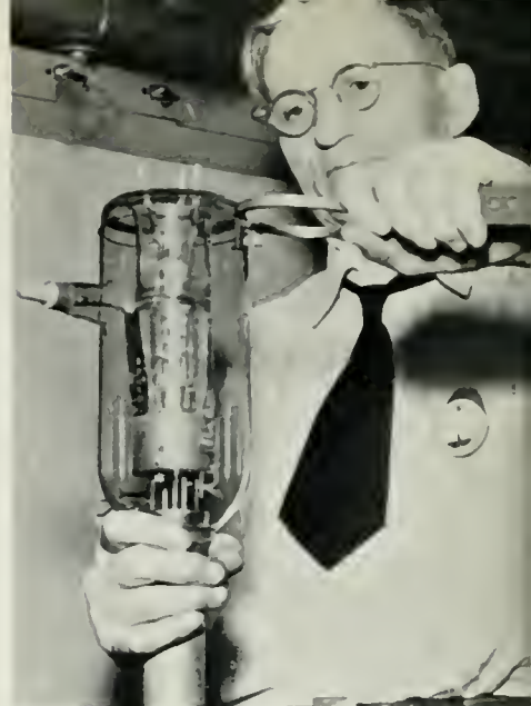
THE FIRST STEP IN REBUILDING AN IN-OPERATIVE POWER TUBE IS TO CUT OPEN THE GLASS BULB, AS SHOWN HERE.
