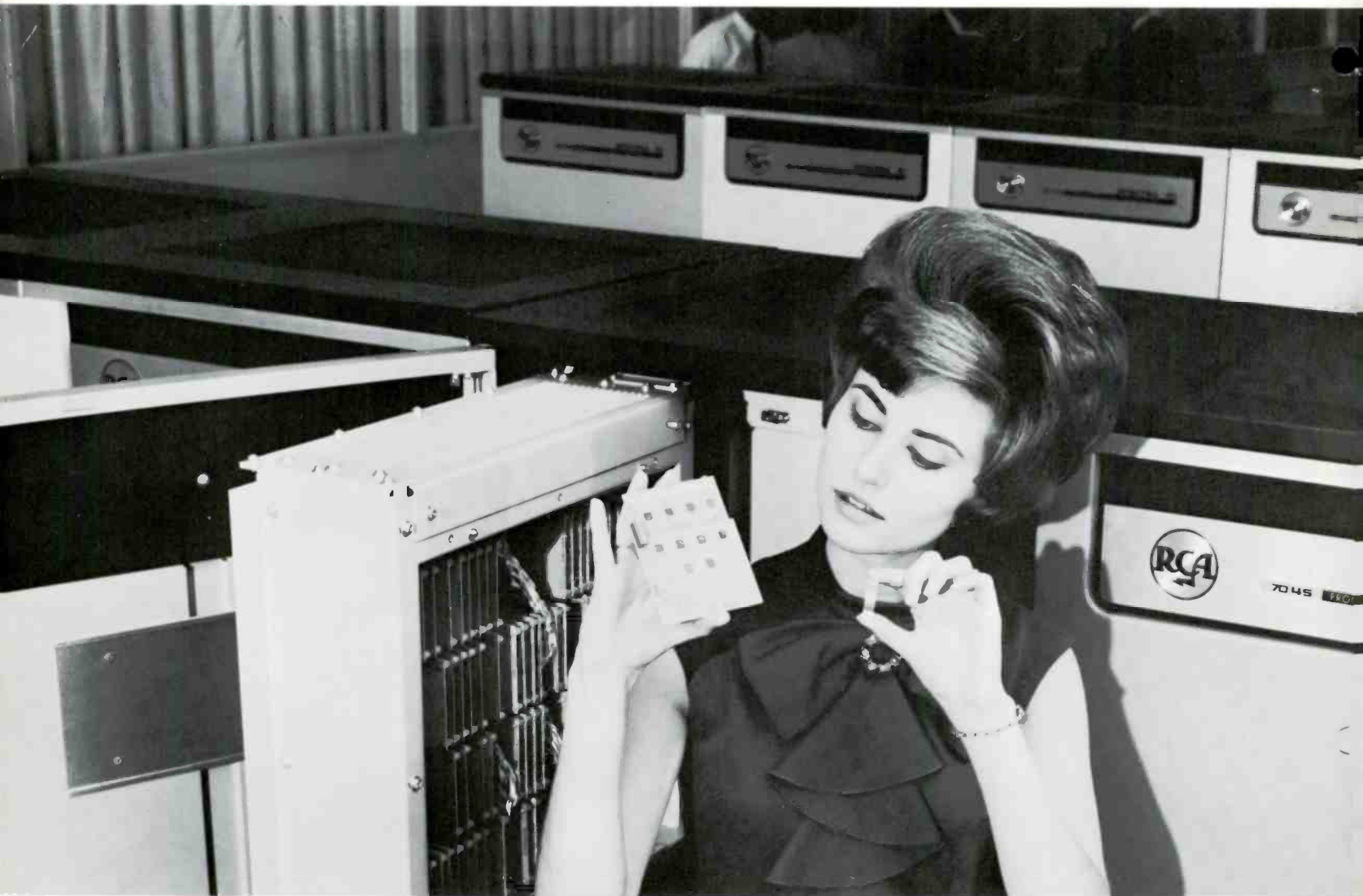
Integrated circuits are packaged into a "flat-pack," which becomes part of a plug-in module used in an RCA Spectra 70 computer.
