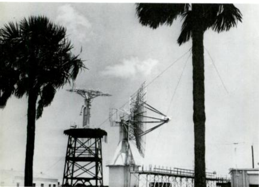
Two telemetry antennas are silhouetted against the Florida sky in the Cape Kennedy launch area.
