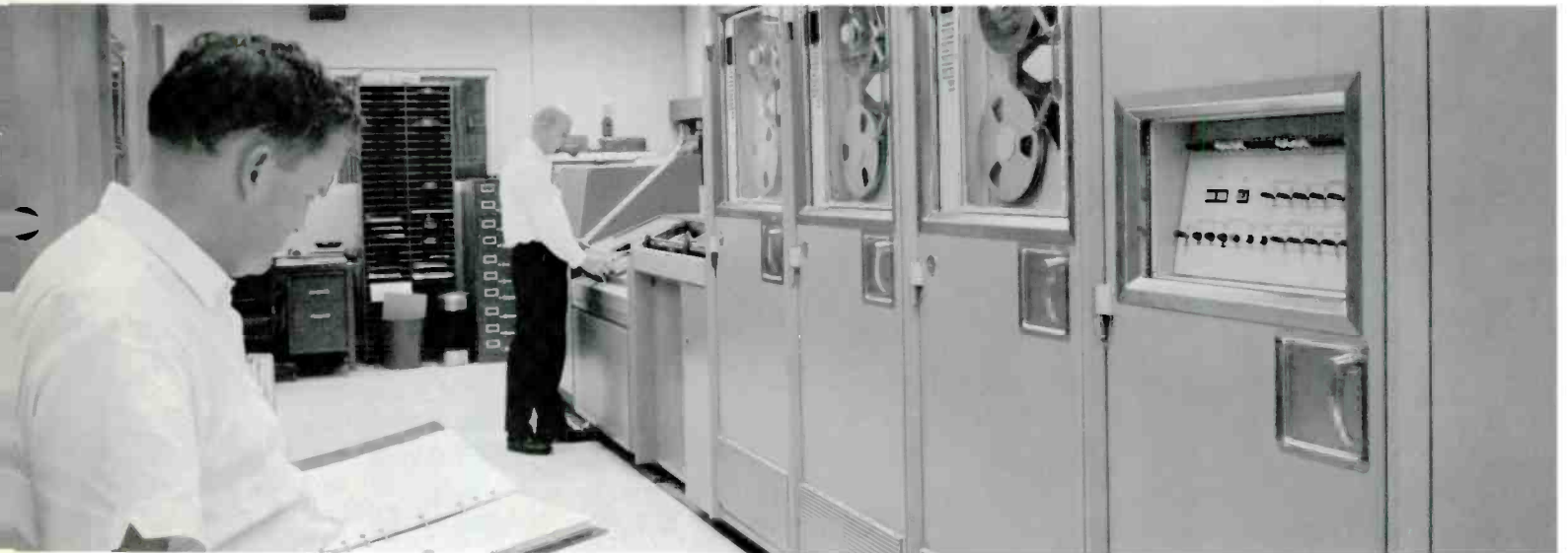
Technicians check one of the 29 RCA 110A computers scheduled for service in NASA's Saturn/Apollo program, including checkout of launch itself.
