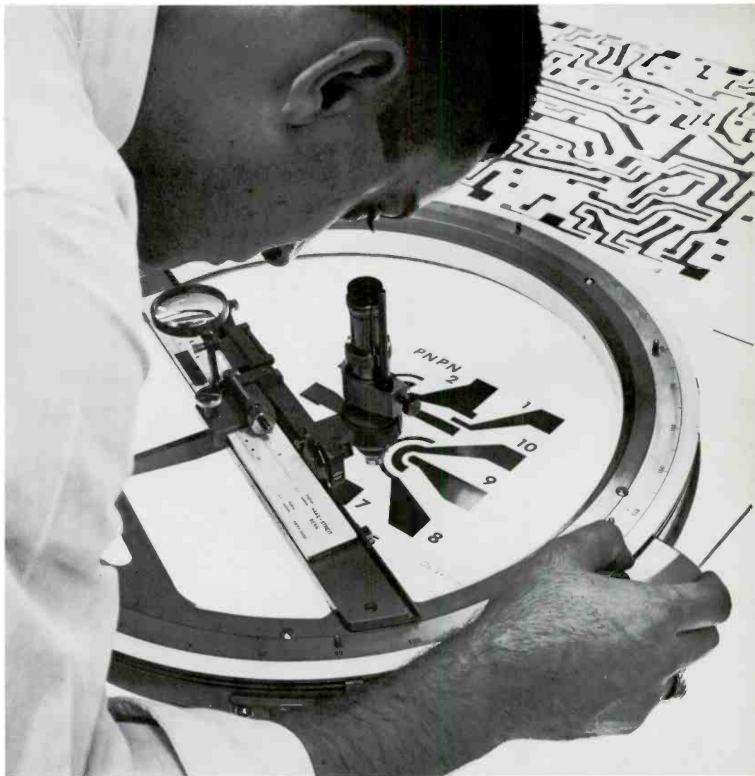
Technician uses microscope to inspect oversized pattern of an integrated circuit.
