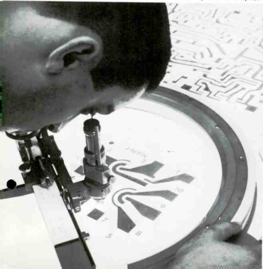
Oversized pattern of an advanced integrated circuit for use in Spectra 70 computer.
