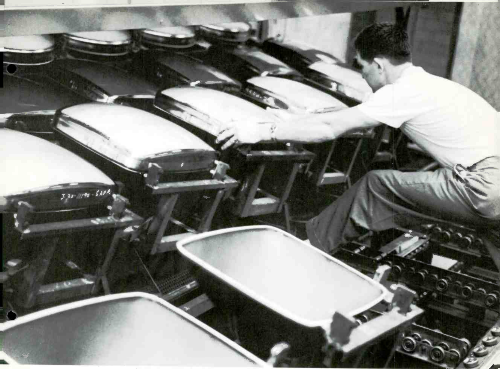
Production of 25-inch color television picture tubes at RCA's Lancaster, Pa., plant.
