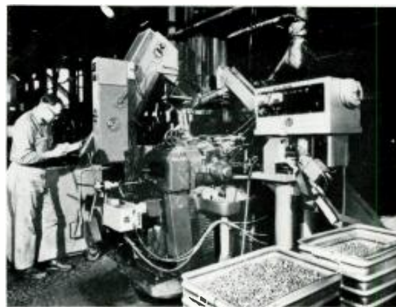
This automatic grinder is one of many electronic controls now in use in the steel industry. It can automatically gage metal slugs and send rejects back through the grinder.
