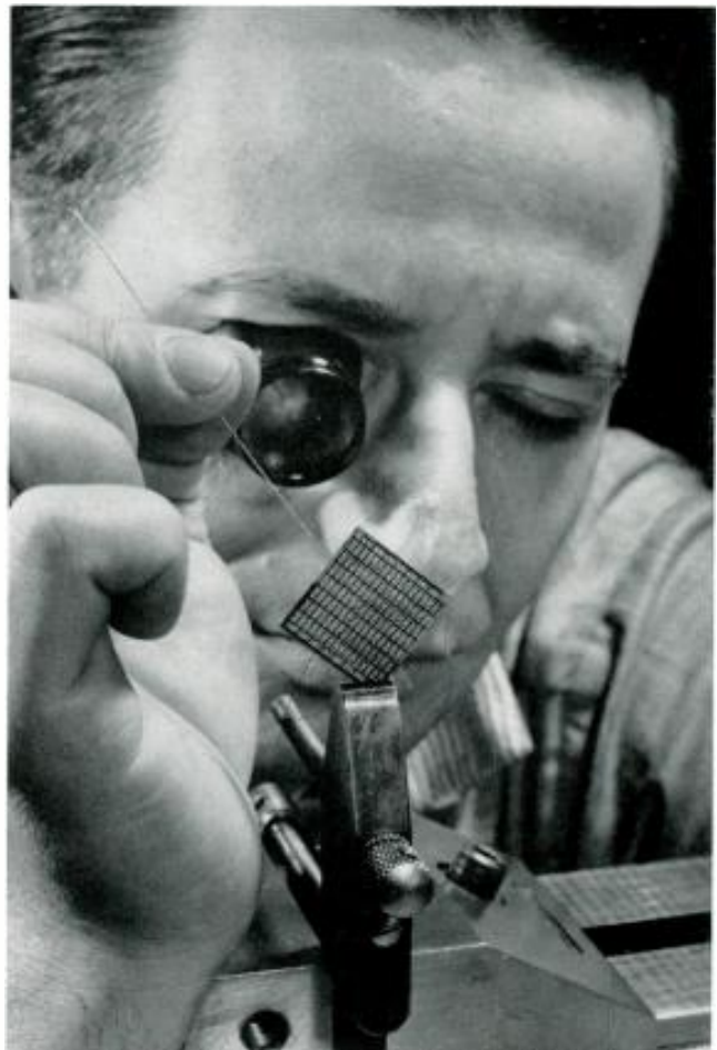
Laboratory technician Claude Wilton of the West Coast Electronics Center carefully threads a tiny grid which can hold 2,200 "bits" of electronic memory. The grid will replace present grids more than 10 times its size.
