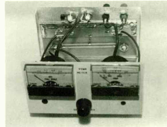
PHOTO 7 The RF coupling lines on the back of the chassis show how the microstrip design is implemented. The 39 ohm matching resistor is the central part of the photo.
