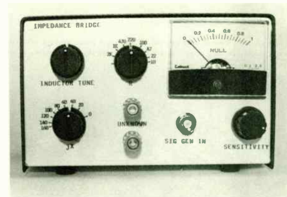
PHOTO 8. The Impedance Bridge will analyze parallel impedances from 20 pf to 10 ohms.
