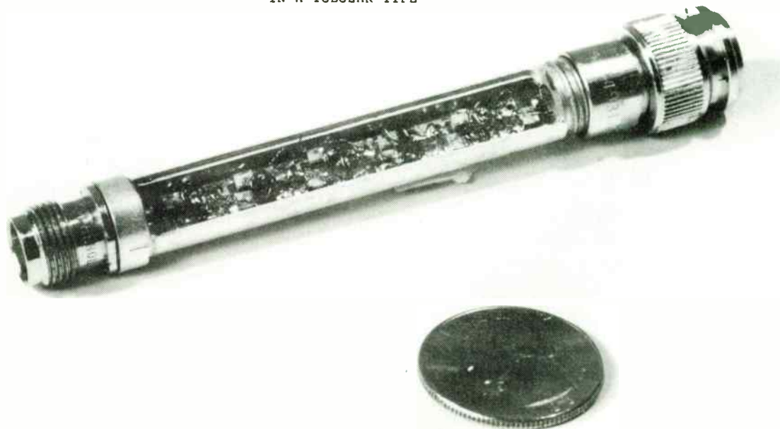
FIGURE 14 LUMPED ELEMENT BANDPASS IN A TUBULAR TYPE
