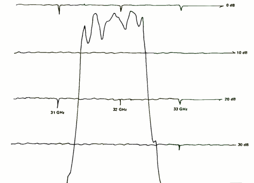
Figure 4. A 1 GHz bandwidth 3 dB ripple Chebyshev filter, designed with a 32 GHz center frequency will produce the above response curves.
