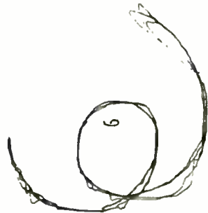
Figure 4. Top plot was made with a Hewlett-Packard 8510 Network Analyzer. The bottom plot is the same load measured with the Impedance Meter. Shapes of the curves are nearly identical, with some differences in rotation of the display and the calibration of the center dot (50 ohm load).
