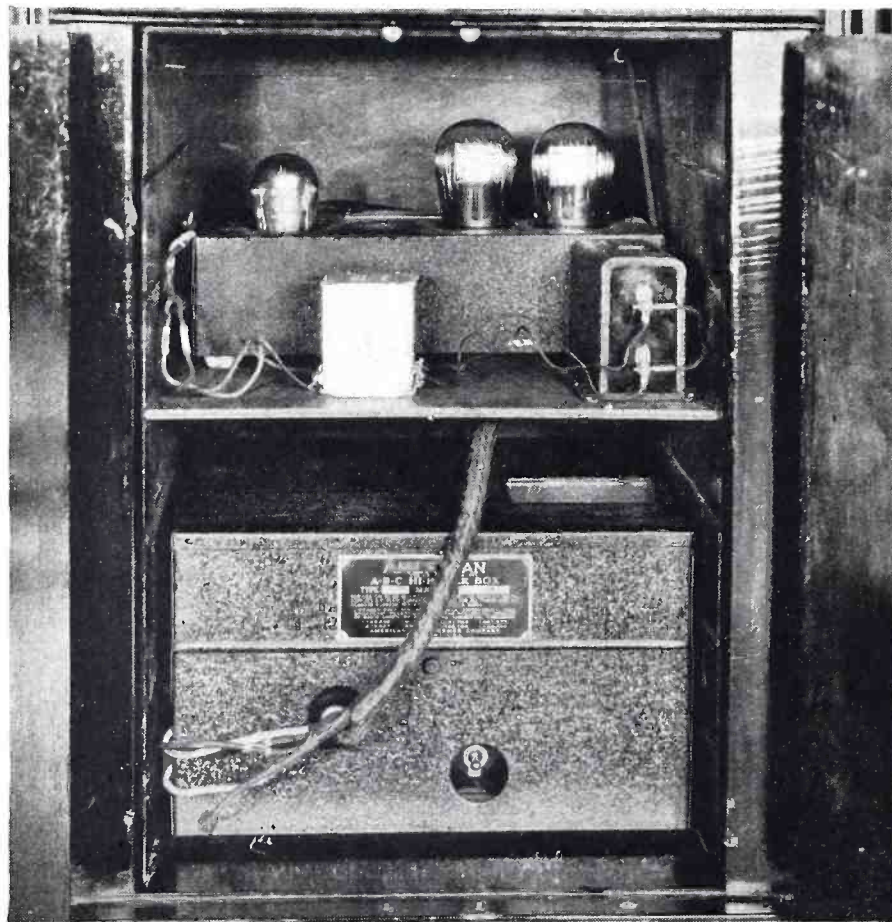
FIGURE 2: The high-power box is placed in the lower part of the cabinet of the phonograph, while the amplifier, the needle-scratch filter, and the impedance balancer are placed on one of the shelves that formerly held the records. The other record shelves are taken out to make room for the instruments.
