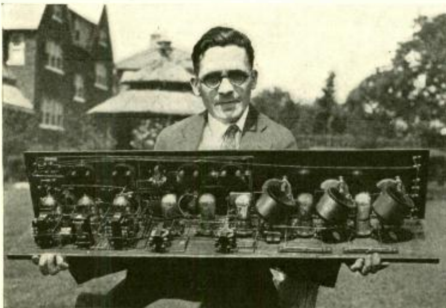
Homemade, tuned-radio-frequency sets, unless they are properly neutralized, may oscillate in one or more stages. If this is the case, this type of circuit may be just as bad an offender as the simple one-tube regenerative receiver.
