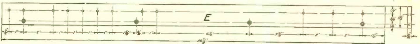
FIGURE 9: This drawing shows the dimensions for the strip and the spacings for the holes that should be drilled to mount the binding posts and the connection strip itself.
