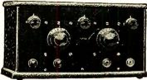
Model C-18 Three-tube Receiver. Gives five-tube volume with only three tubes, due to reflex amplification. Finished in black leatherette.
