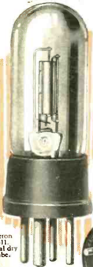
Radiotron WD-12. The standard base dry cell tube.
