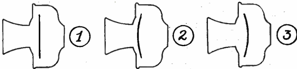
FIGURE 3: This diagram shows how the electric current that flows through a microphone varies with the strength of the sound waves. The currents for the three positions of the diaphragm shown in Figures 1 and 3 are indicated.
