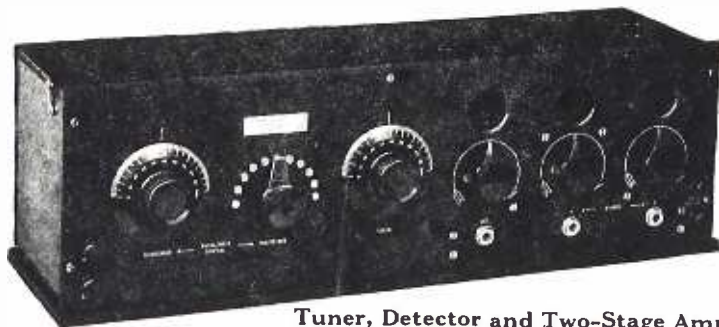
Tuner, Detector and Two-Stage Amplifier Type 115
