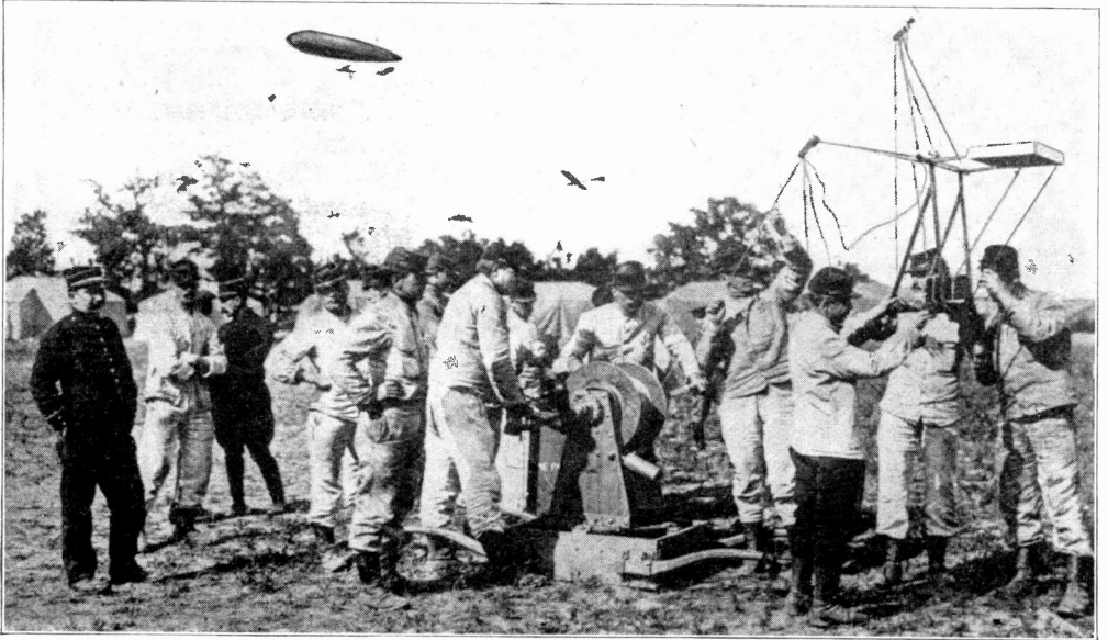
PORTABLE GROUND STATION USED IN CONNECTION WITH AEROPLANE WIRELESS EXPERIMENTS
